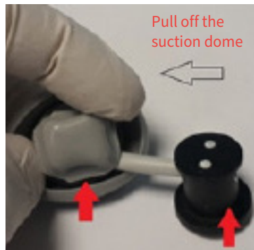
Diagram 9: Remove the suction dome
