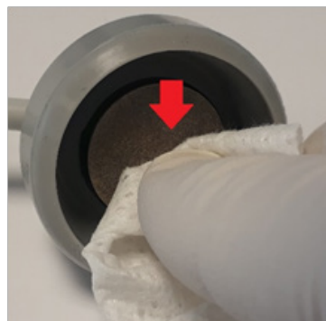
Diagram 2: Clean contact surfaces
