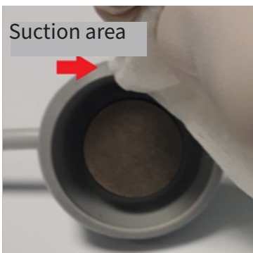
Diagram 6: Suction dome cleaning outside
