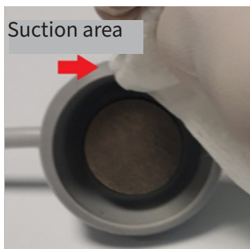
Diagram 1: Suction dome cleaning outside
