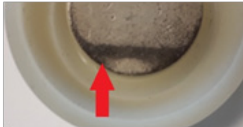
Diagram 14: Error image - discolouration of the electrode
