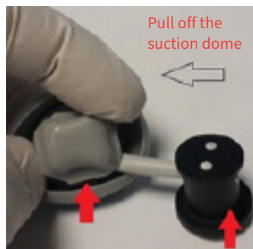
Diagram 11: Remove the suction dome
