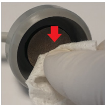
Diagram 7: Clean contact area (electrode)
