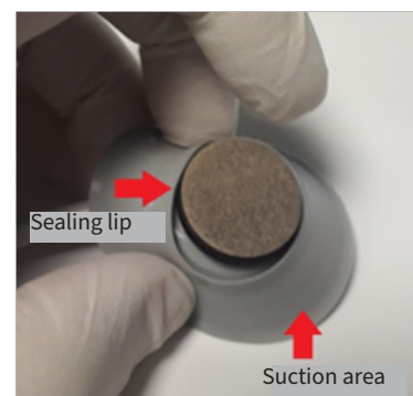
Diagram 8: Suction dome cleaning inside
